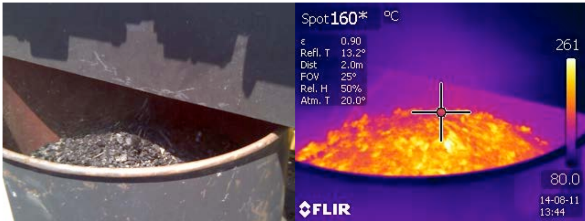
Figure 24. Infrared image of biochar collection with temperatures up to 261°C.
