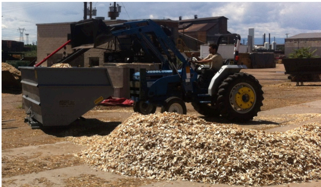
Figure 4. Loading feedstock into the self-dumping hopper to prepare for SS operation. A small feedstock pile is shown in the lower portion of the image.
