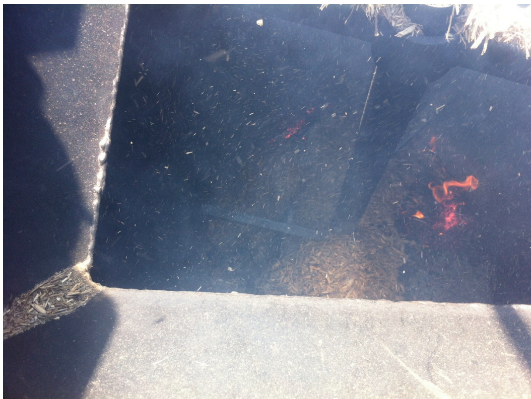
Figure 23. Picture from top of reactor looking downward. Notice the flame front extending upwards and dust suspended in the air. Biomass also collects on the top of the stir bar and the corners of the reactor inlet as seen in the top right and bottom left of the picture, respectively.
