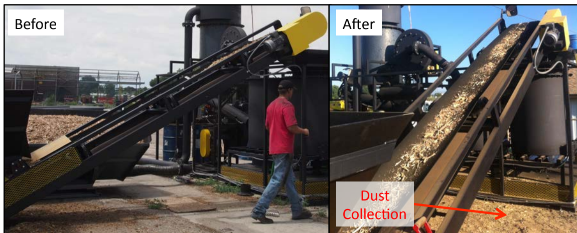
Figure 22. Dust collection around the conveyor after three weeks of use.
