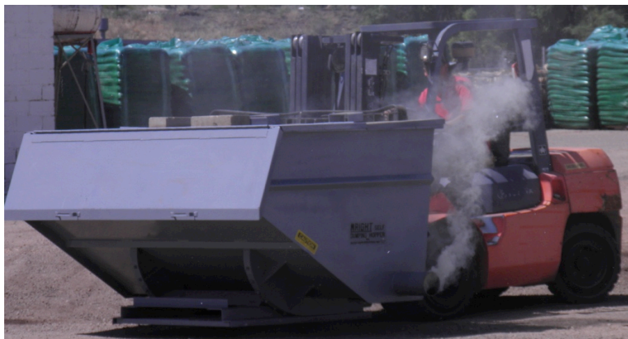
Figure 25. Dryer hopper being transported away from the biochar production machine after combustion started. Notice the smoke rising from the air inlet port.
