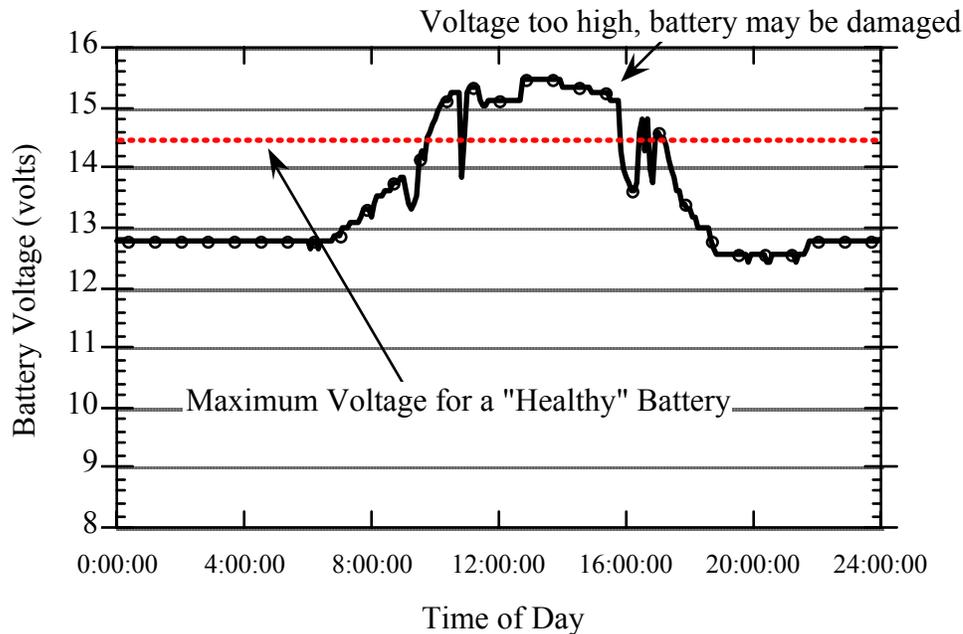
**Figure 1: Battery Voltage versus Time of Day for a 36 Watt Solar System in Kenya; the system does NOT include a charge controller.**
