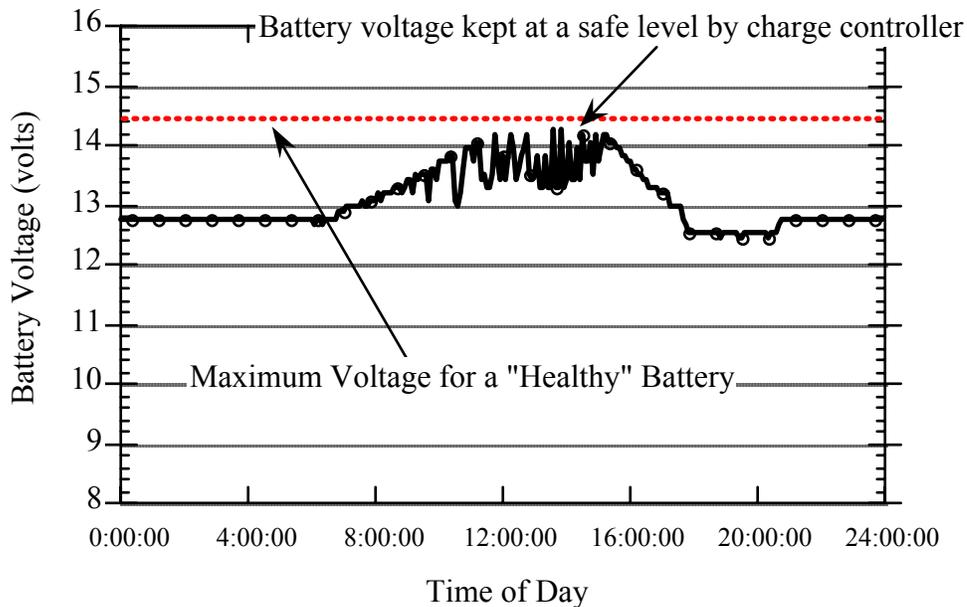
**Figure 1: Battery Voltage versus Time of Day for the Same 36 Watt Solar System after a Charge Controller Was Added.**
