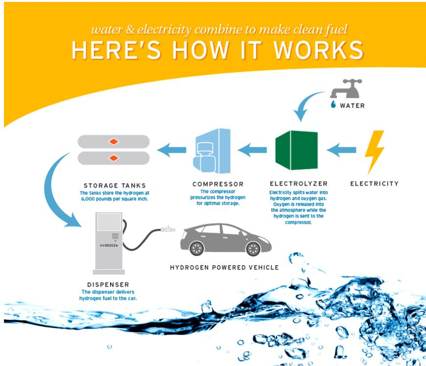
**Figure 3.** An interpretive sign at the HSU Hydrogen Fueling Station that describes the hydrogen generation process to visitors.
