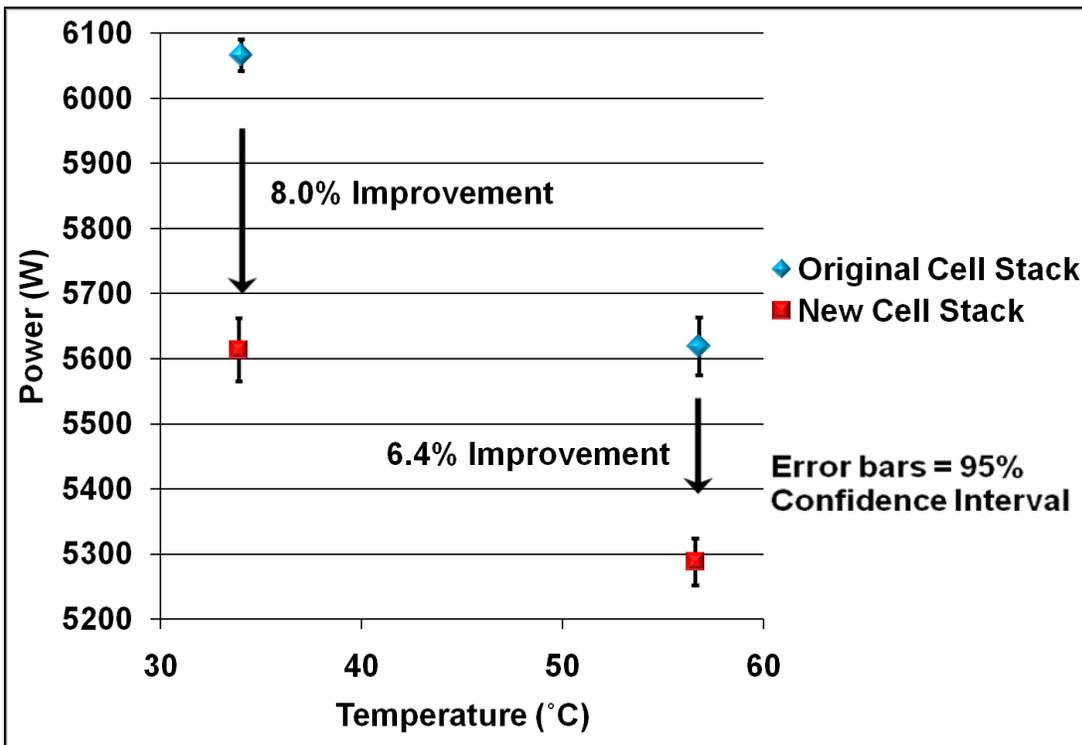
**Figure 7. Power consumption of cell stacks at 34°C and 56°C**
